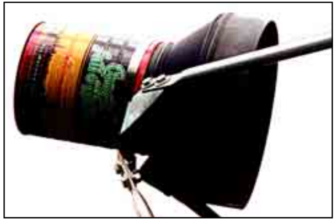
Since we intend to use the VSA at L-band, on a frequency of 1296 MHz, one can scale the dimensions of the standard C-band feed by a factor of three. As is the amateur tradition this feedhorn is constructed from low-cost materials!
