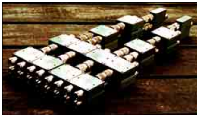
The VSA phasing matrix. These bias Ts and power dividers/combiners will produce four different beam patterns simultaneously, in two orthogonal circular polarizations.
