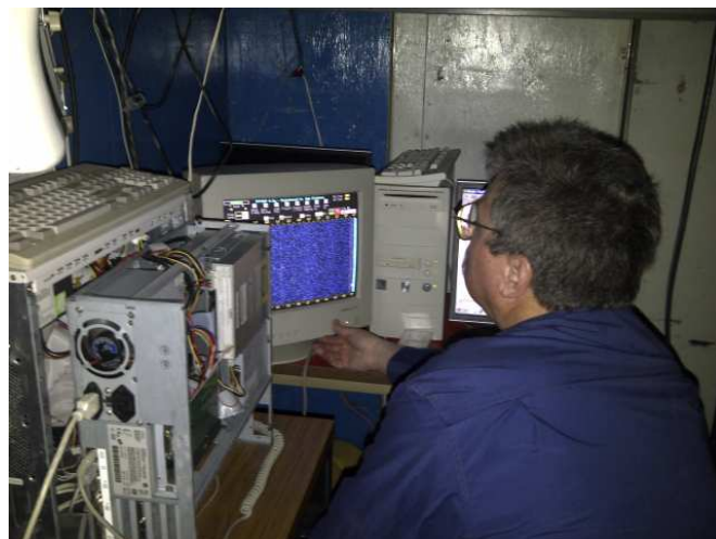
FIGURE 3: ROBERT STEPHENS ANALYZING THE STEPHENS MYSTERY SIGNAL ON AN FFT-DSP WATERFALL DISPLAY
