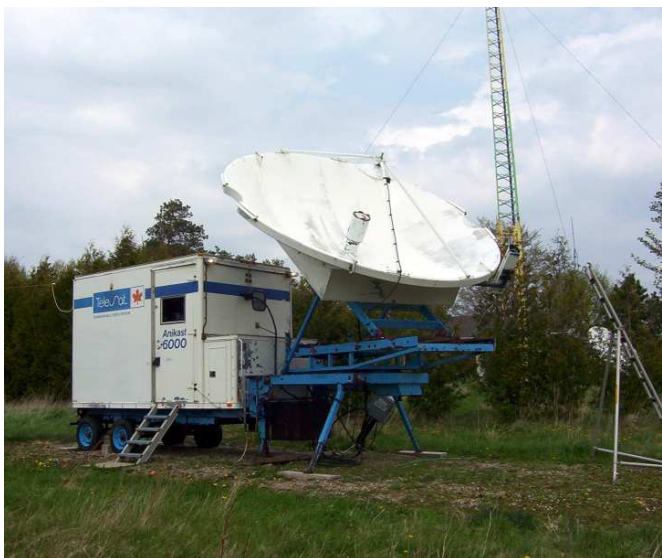
FIGURE 1: THE 4 GHz, 4.5 METRE RADIO TELESCOPE AT ROBERT STEPHENS' AREA 31 RADIO OBSERVATORY IN CANADA
