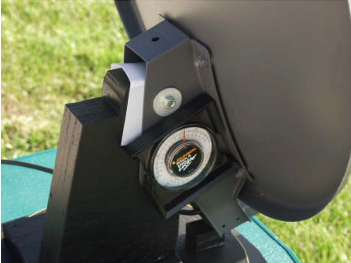
The readout will not be accurate, but the experiment below will help you determine the correction factor. Hot plastic glue holds the protractor to the dish just fine.
