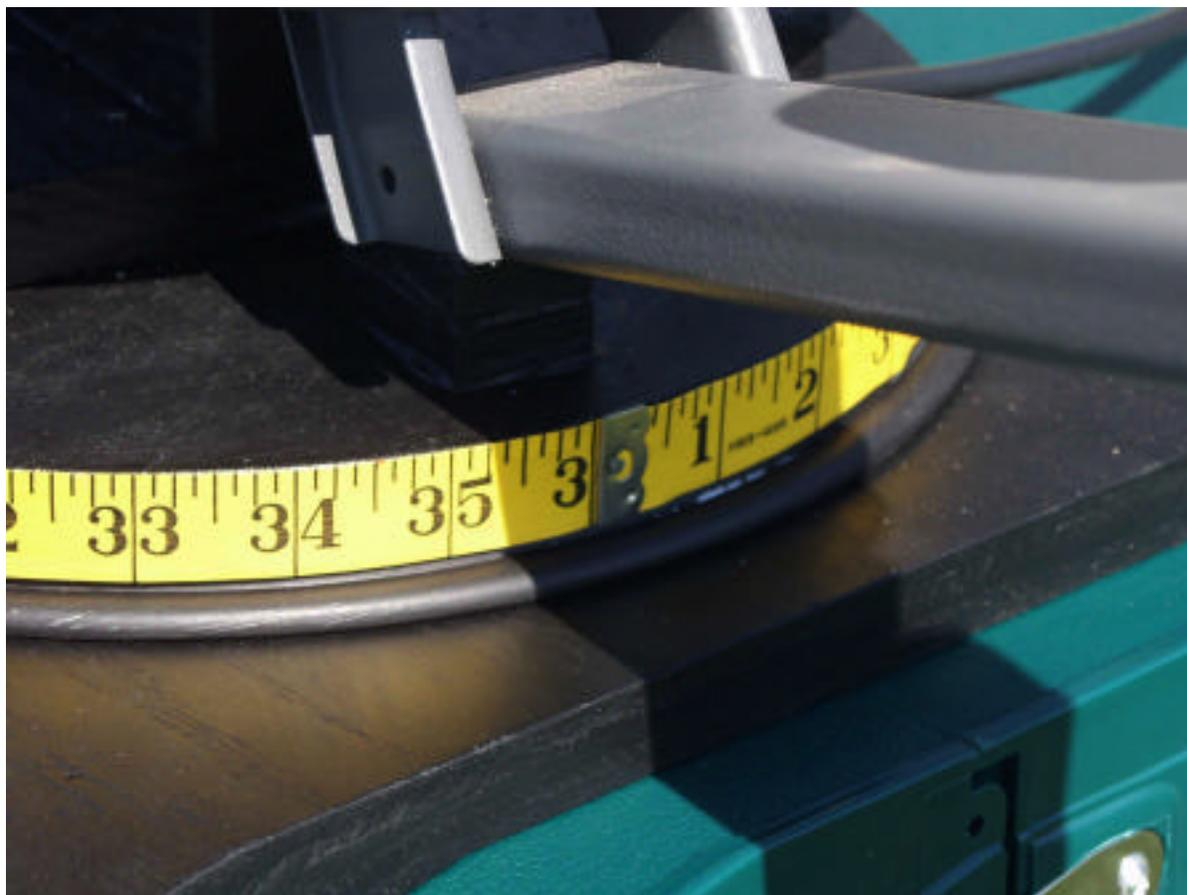
A \$6.00 rotary protractor at the builders store provides the elevation readout.
