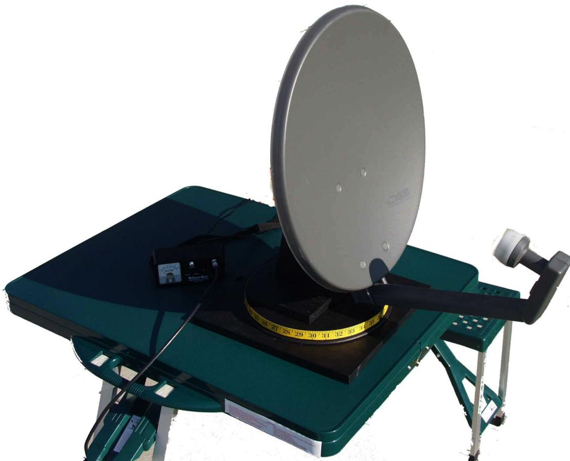
A simple RF/IF/Detector unit is a Channel Master Model 1004IFD tuning meter that includes an **audible tuning indicator**.
