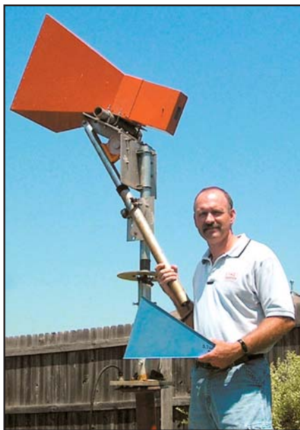
Tommy Henderson, WD5AGO, shows off two horn antennas used for radio astronomy. The larger of the two (on an az-el mount) is optimized for 1.4 GHz hydrogen line observations. Tommy is holding a smaller horn for 5.7 GHz methanol line measurements.
