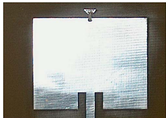
Figure 6 ATDM-loaded microstrip antenna element
