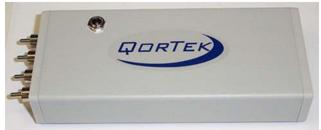
Figure 9 High-voltage driver amplifiers (packaged)
