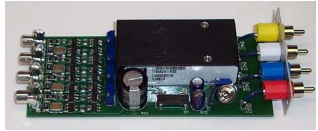
Figure 8 High-voltage driver amplifiers (circuit board)
