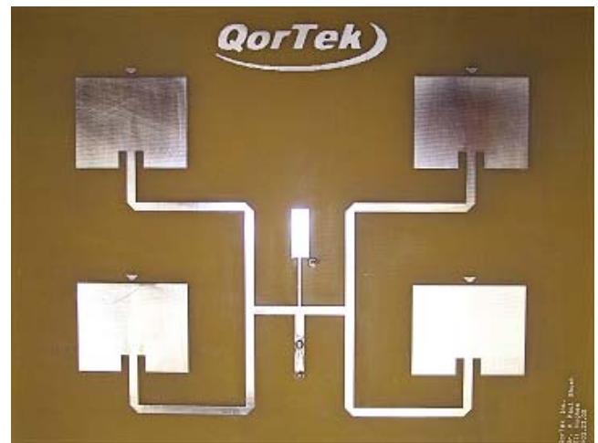
Figure 1 Typical microstrip phased array antenna
