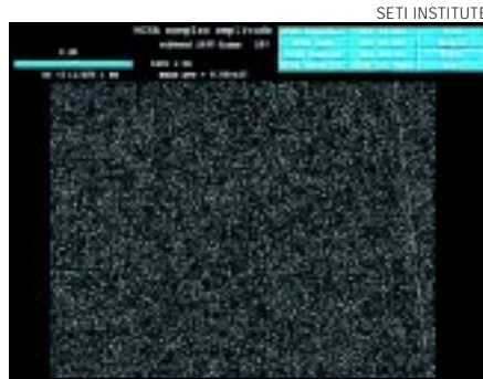
Figure 4—Pioneer 10 beacon as received at Arecibo, displayed on the Project Phoenix spectrograph (faint trace on right side of screen).
