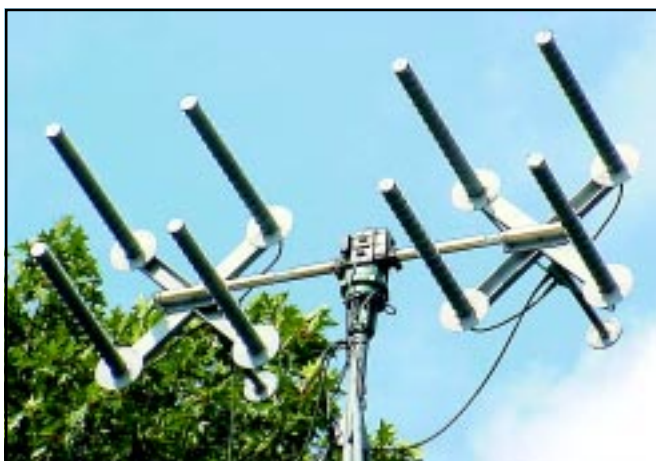
Figure 11—EME beacon antennas: four RHCP and four LHCP helices.
