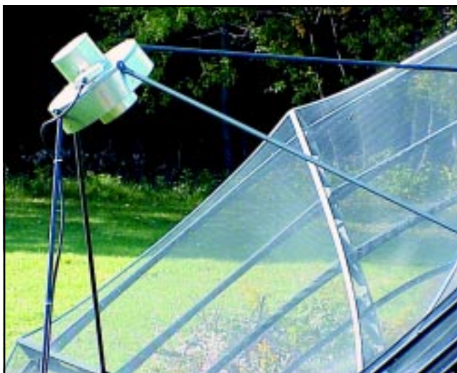
Figure 1—A typical hydrogen-line radio telescope.
